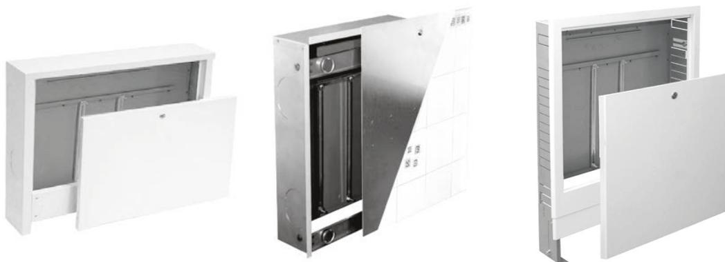
Due to the design of cabinets for floor heating manifolds can be mounted with or without a mixing device. In cabinets there is also room for electrical terminal blocks. Terminal blocks are attached by screws, which enter into special holes in a mounting strip in the upper part of a box.
