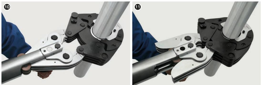
10 **Assembling the machine to the jaw**
