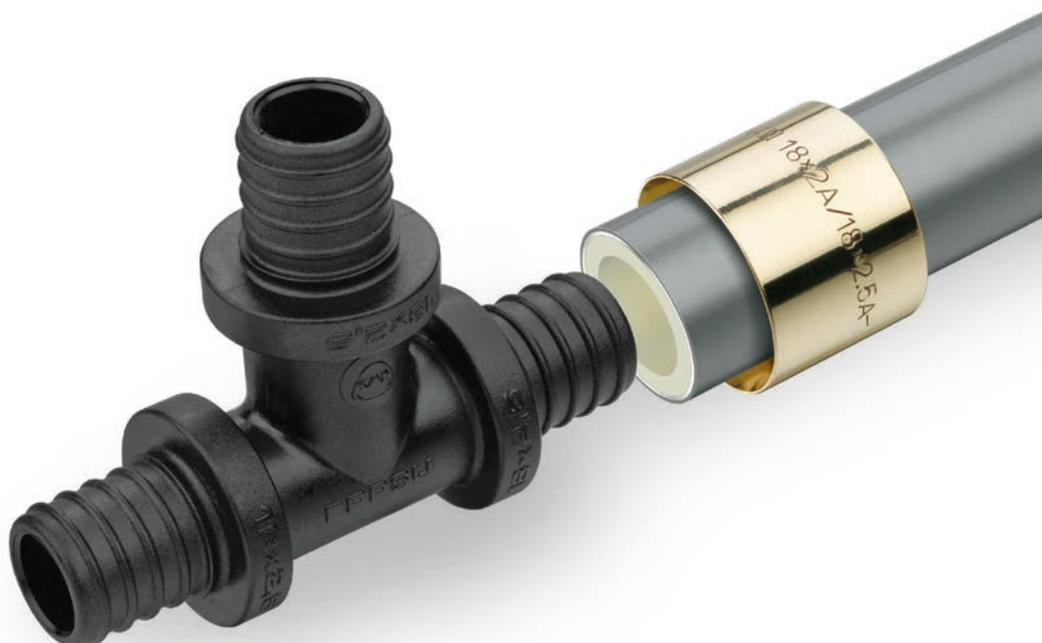
Push Platinum System leak-tight joints without O-Rings are made by pushing a brass sleeve onto a fitting and a pipe. These connections do not require additional sealing like a PTFE tape or tow. The system is complemented by manifolds and installation cabinets available in section Manifolds, cabinets and accessories.
