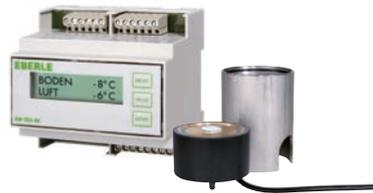
**A controller of open space surface ice formation** – with a sensor of snow and ice cooperating with a heating system protects from ice formation and snow accumulation on traffic courses (external stairs, sidewalks, parking places, drives etc.).
