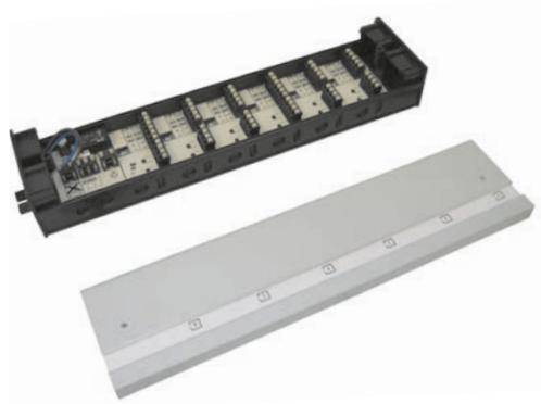
The Basic terminal block for heating and cooling with a pumping module in a 230V and 24V version allows to connect thermostats and actuators at one place in an installation cabinet (above a manifold). Maximally you can connect 6 thermostats and 12 actuators.
