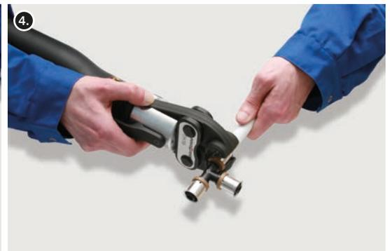
5. Start the press drive and make the connection. The process of pressing lasts till the jaws close fully. The ring can be pressed on a pipe only once.
