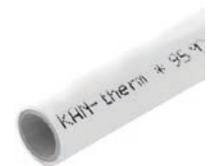
multilayer pipe PE-Xc/Al/PE-Xc (PN12 series) designed for central heating, hot and cold water systems as well as for underfloor heating systems; operating pressure max. 10 bar
