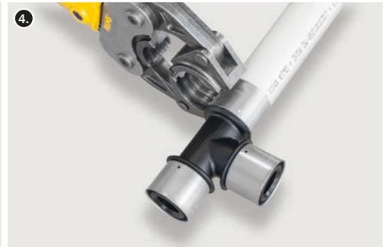
5. Apply the clamping tool jaws on a ring so it contacts the tube coupling collar. The external collar of jaws shall be pushed to the tube coupling collar but not embrace it. Start the clamping tool drive and make the connection.
