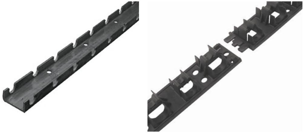
Mounting rails are equipped with adhesive tape and can be fastened to foamed polystyrene boards Tacker or directly to the base. Applying pipes of  $\text{Ø}12 \times 2$  and  $\text{Ø}14 \times 2$  mm in diameter fastened to mounting rails works perfectly in wall heating designs where pipes mounted in walls are covered with a layer of special plaster.
