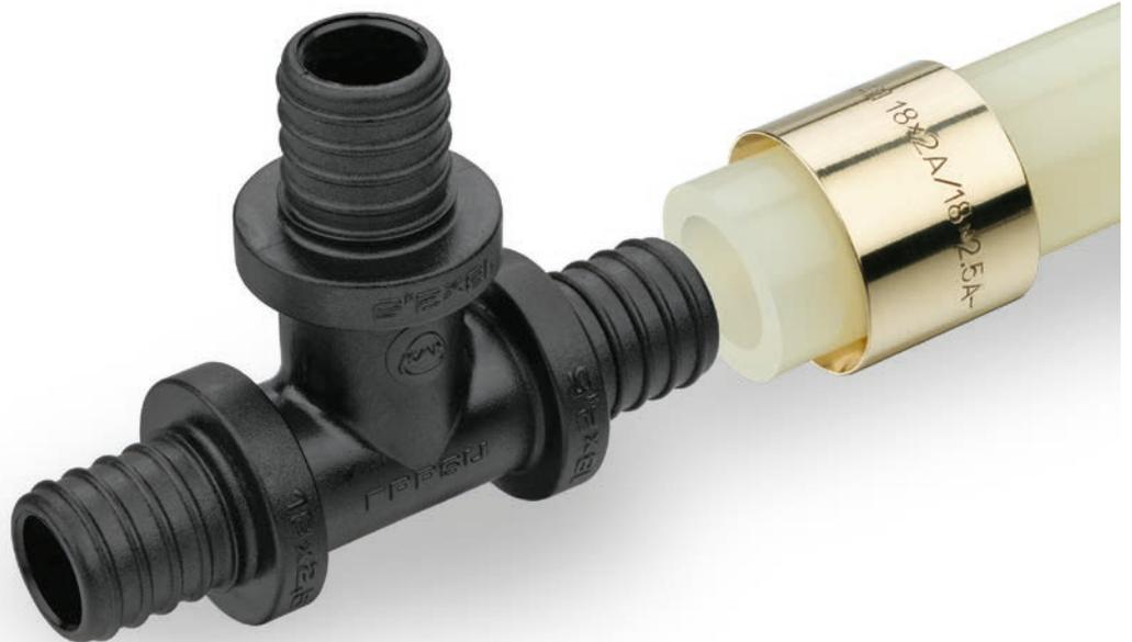
A KAN-therm Push System leak-tight joints without O-Rings are made by pushing a brass sleeve onto a fitting and a pipe. These joints do not require additional sealing like a PTFE tape or tow. Other complementing elements of the system are manifolds and installation cabinets.
