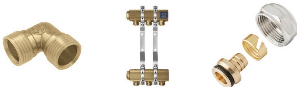
Eurocone adapters are characteristic for a sealing on the cone and an O-Ring between body and a fitting. This kind of joints is self-sealing and no additional sealing element like a PTFE tape or tow shall be used. Locate such connections at generally accessible places.
